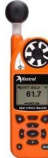
**Hand-held device that estimates wet bulb globe thermometer**
