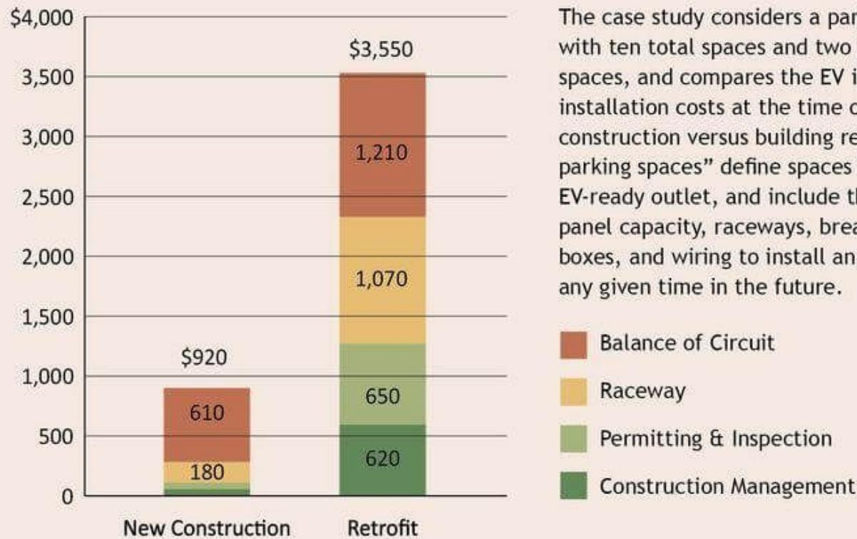
The case study considers a parking lot with ten total spaces and two EV parking spaces, and compares the EV infrastructure installation costs at the time of new construction versus building retrofit. "EV parking spaces" define spaces that have an EV-ready outlet, and include the electrical panel capacity, raceways, breakers, outlet boxes, and wiring to install an EV charger at any given time in the future.
