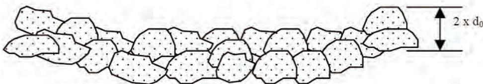
**Riffle Section through Cobble**
